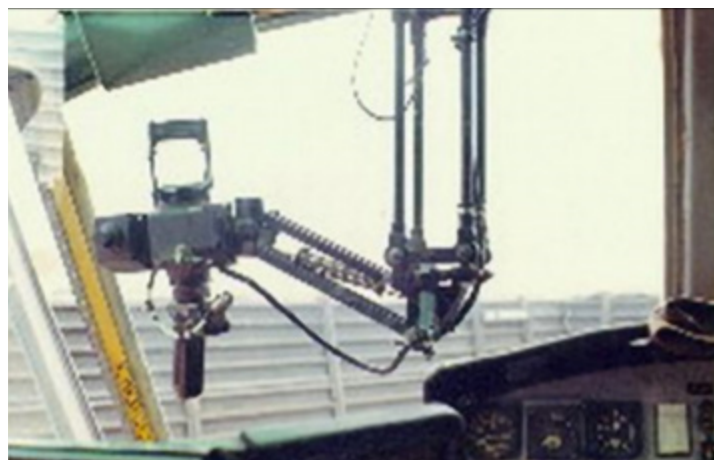
In the photo above, minigun sight that remotely controlled the guns. The lower handle had the trigger on the top and below was a trigger that activated the movement of the gun to point at the target.
