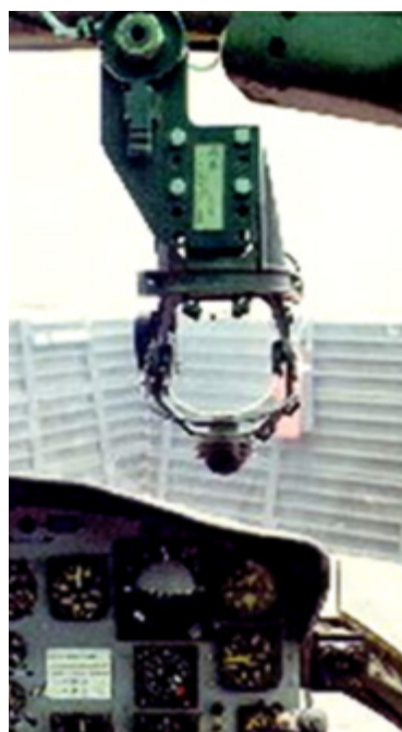
In the photo at left, the rocket sight in the down position.
